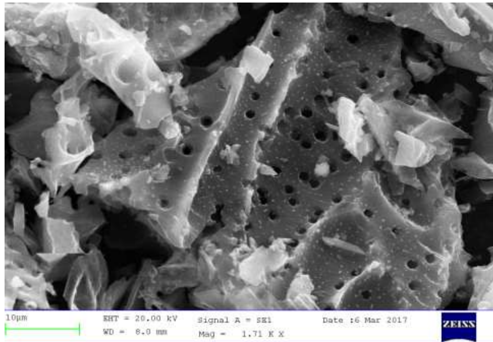
Figure (3) SEM Image of Groundnut Shell Carbon before Activation
